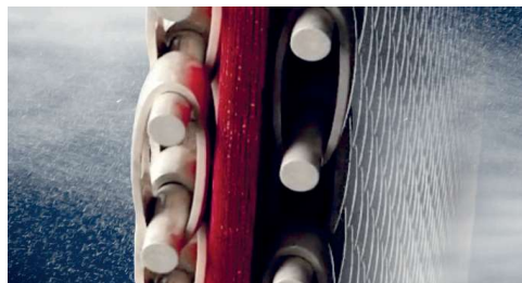
↑ Kinetika is used for the processing of particularly fine and delicate fabrics and for high-density fabrics (Biella Shrunken Process).
