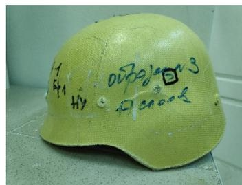
Helmet made of prepreg based on aramid fiber and thermoplastic binder
