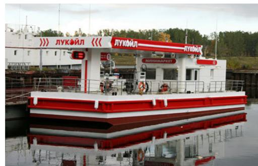
Non-self-propelled floating gas station
